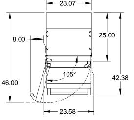
NOTE: A 90°DOOR OPENING IS SUFFICIENT TO ALLOW FULL EXTRACTION OF THE INNER DRAWERS, EVEN IF THE APPLIANCE IS DIRECTLY ADJACENT TO A WALL. HOWEVER IF 105°OPENING IS DESIRED, THEN POSITION APPLIANCE AT 8" DISTANCE SHOWN.
